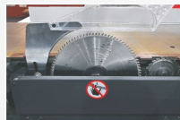
Saw Unit • High precision cutting. • Main saw RPM 4000/6000 • Noise less standardized motor. • Easy up-down of main saw and scoring saw. • Left & right movement of scoring saw.
