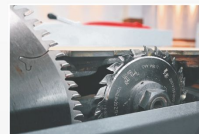
Scoring Unit • With high RPM : 8000 • Scoring unit helps to cut a laminate or any type of wood beneath. • Burr free cutting. • The scoring saw blades rotate in the opposite direction to the main saw.
