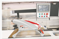
N.C. Controlled Rip Fence • Error Less accurate movement of rip fence • Controlled by servo motor • Serial Movement Can be performed by just one touch according to PLC data list
